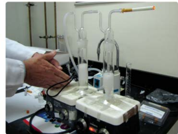
Air is drawn through an e-cigarette during a laboratory procedure that simulates a smoker taking a puff. The resulting vapor is tested.
