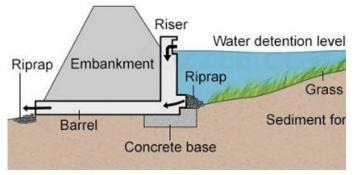
Unless there is a lot of rain, detention ponds are normally dry. They're made to temporarily store water before slowly draining it to another site. but they also aid in the slowing of runoff, the containment of silt, the collection of rubbish, and the removal of contaminants.
