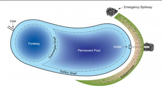
An inlet delivers runoff from streets and other areas, and the outlet structure allows the pond to fill and gradually drain. Accumulated sediment and associated pollutants are stored in the bottom of the pond for periodic removal and disposal.
