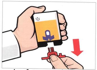
Note: the red safety guard is made to fit firmly to remove.
